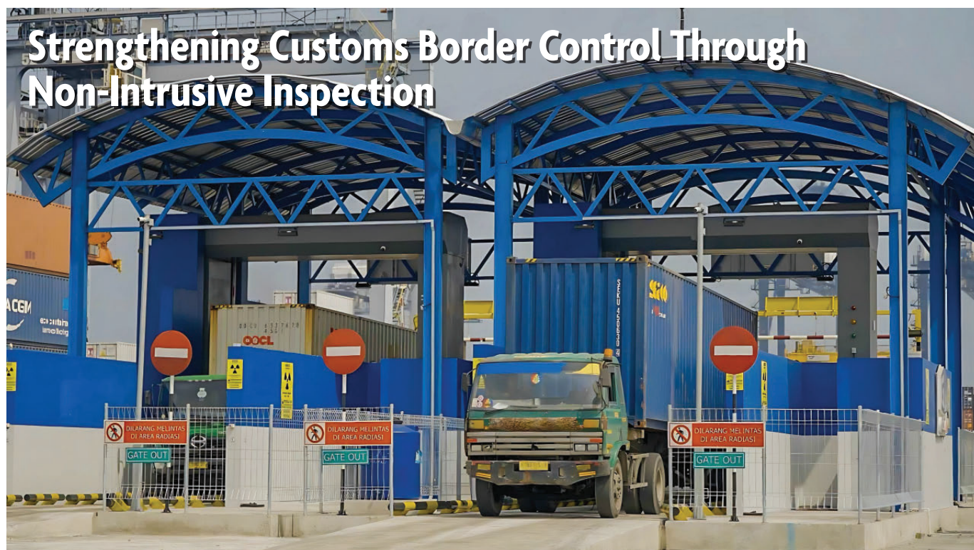
Container trucks pass through x-ray container scanners at PT Jakarta International Container Terminal, Port of Tanjung Priok, North Jakarta, Indonesia.
